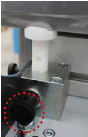
Fig. 12: Setting rear panel heights
