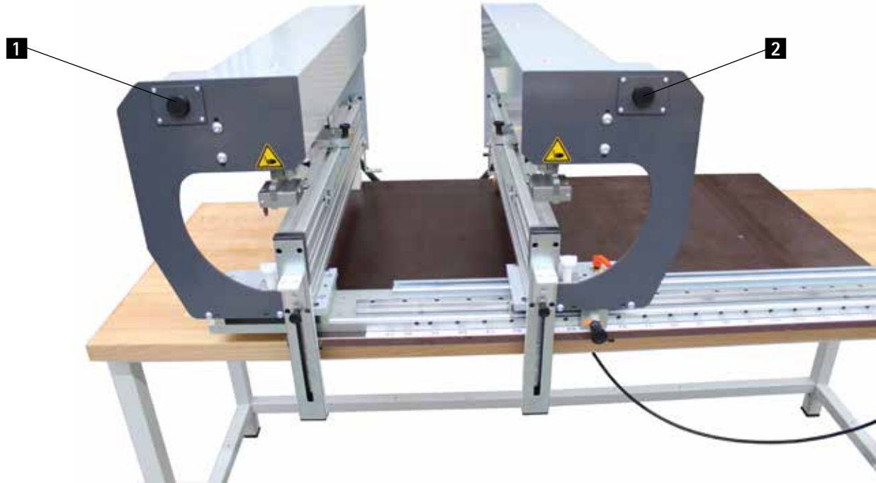
Fig. 4: Two hand switch system
