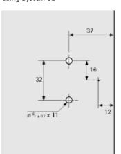
For overlay doors, for hinges using System 25
