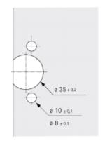
Production tolerances shown in the drawing must be kept.
