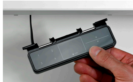
Fig. 34: Control panel detached from above from its anchorage
