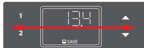
Fig. 49: The LegaDrive Touch Inlay handset lock is activated and deactivated by swiping to the left or right
