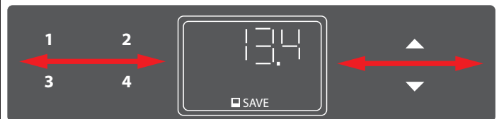
Fig. 48: The LegaDrive Touch Comfort handset lock is activated and deactivated by swiping to the left or right
