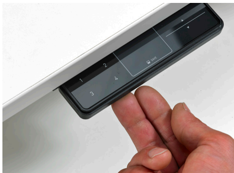
Fig. 32: Lifting and pushing the control panel to retract it
