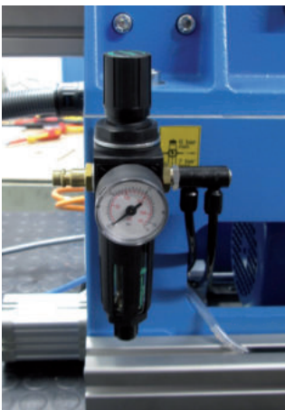
Fig. 5: Compressed air connection
