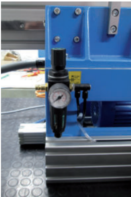
Fig. 5: Pneumatic system servicing unit (viewed by the operator, on the left hand rear side of the machine frame)
