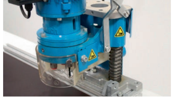
Fig. 4: Sliding guard at drilling spindles
