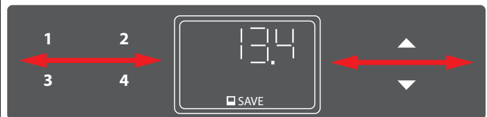
Fig. 50. The LegaDrive Touch Comfort handset lock is activated and deactivated by swiping to the left or right
