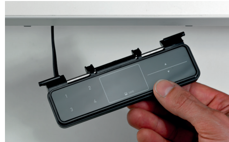
Fig. 35. Control panel detached from above from its anchorage
